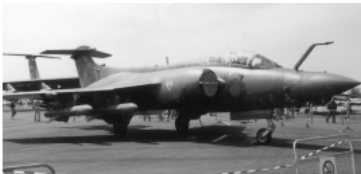
Fig 3-2 Area Rule- 'Coke-Bottle' Fuselage Photo: R Wilkinson
