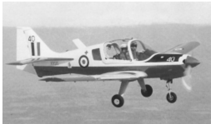
Fig 8-1 two Main-Wheels and a Nose-Wheel
